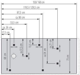
IMPORTANT! The dimensions of the casing must be observed exactly! The tub can be set exactly 14 cm lower!
